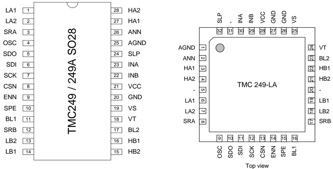
Note: Cooling plane on -LA type should be connected to GND or left open.
