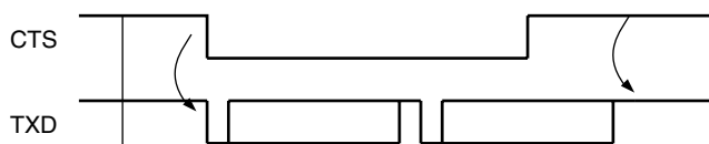
Figure 30-19. Transmitter Behavior when Operating with Hardware Handshaking
