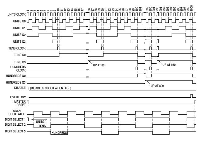
Figure 1. 3-Digit Counter Timing Diagram (Reference Figure 3)
