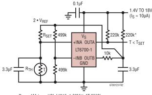
$R_{TH}$  = 1M (e.g., YSI 44015, 1.00M $\Omega$  AT 25°C)  $R_{SET}$  =  $R_{TH}$  AT  $T_{SET}$  \*RESISTANCE MAY REQUIRE OPTIMIZATION FOR OPERATION OVER INTENDED  $R_{TH}$  AND  $V_{SUPPLY}$  RANGES HYSTERESIS ZONE  $\approx$  0.4°C
