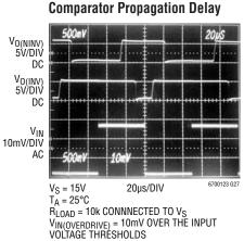
Noninverting and Inverting
