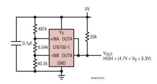
Figure 1. Simple Window Comparator
