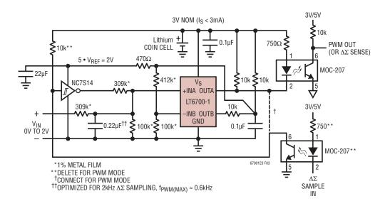
Figure 3. Isolated PWM or  $\Delta\Sigma$  Converter
