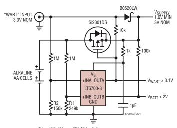
$R1 = 400k/(V_{BATT} AT LOW - 0.4)$  $R2 = 400k/(V_{BATT} AT MAX - 0.4)$
