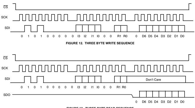
FIGURE 13. THREE BYTE READ SEQUENCE
