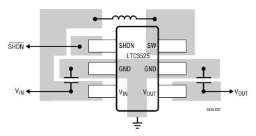
Figure 2. Recommended Component Placement
