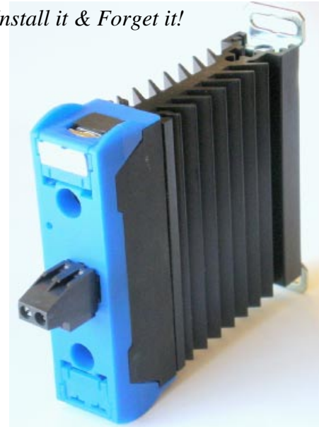
SUL865070= SU865070 SSR + WF311100 heatsink
