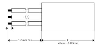
AMPOHM Delta Suppressors are designed for the interference suppression of small motors, business machines and a wide range of domestic appliances in the broadcast band from 20Khz to 3Mhz.
