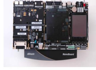
The NanoBoard NB2 provides application-specific plug-in peripheral boards to give complete flexibility in
