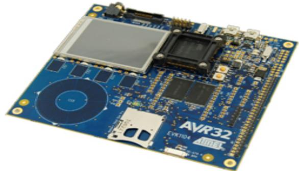
The AVR32 EVK1105 is an evaluation kit for the AT32UC3A0512 which demonstrates Atmel's state-of-the-art AVR32 microcontroller in Hi-Fi audio decoding and streaming applications.
