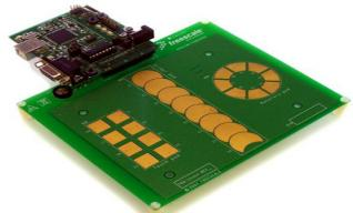
The KITPROXIMITYEVM does not ship with a The KITPROXIMITYEVM does not ship with a MCU development board MCU development kit. For more information on MCU development kits, please refer to the Freescale Development Tool Selector Guide (SG1011).
