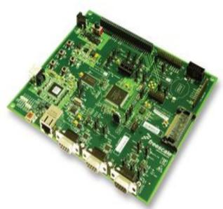
The MCF5225x family consists of highly integrated devices with on-chip USB, Ethernet, CAN and encryption functions, featuring the complete Freescale MQX RTOS software at no additional cost. This solution is ideal for factory automation, building control, and medical applications.
