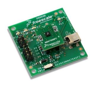
for fast system prototyping and device evaluation within the user's application. This sensor daughterboard is also available in the RD3803MMA7660FC development kit that includes the daughterboard along with the MCU communicator board.
