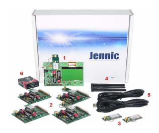
Out of the box, the hardware nodes are pre-programmed and demonstrate an example home sensor demo that monitors the state of sensors on the wireless nodes and presents this information on the controller node's LCD display.
