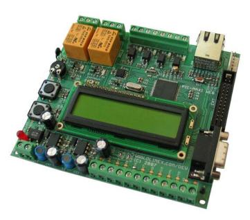
for data storage. The on board DC/DC converter makes this board very tolerant to the external power supply which could be in 9-25V DC or 7-18V AC range. The bridge rectifier on the input allows AC and DC adapters to be used and makes power supply polarity problems go away.
