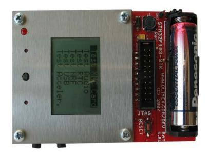
The STM32F103 Performance Line family has an embedded ARM core and is therefore compatible with all ARM tools and software. It combines the high performance ARM Cortex-M3 CPU with an extensive range of peripheral functions and enhanced I/O capabilities.
