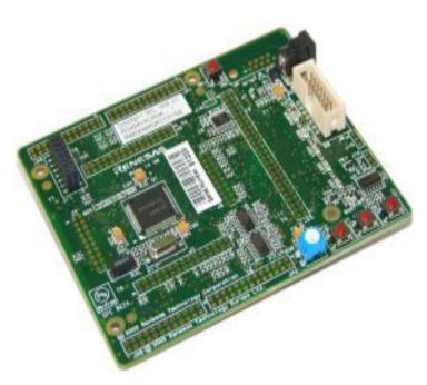
The purpose of the board is to enable the user to evaluate the capabilities of the device and its peripherals by giving the user a simple platform on which code can be run only minutes from opening box. It can also prove an invaluable tool in development by providing a useful test platform for code already debugged using one of our more powerful emulation tools.
