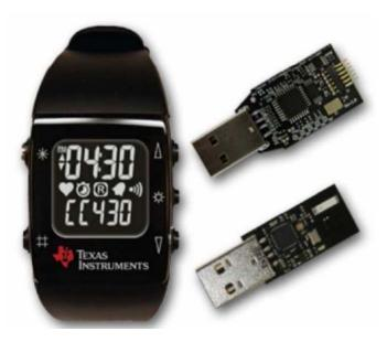
wireless feature allows the Chronos to act as a central hub for nearby wireless sensors such as pedometers and heart rate monitors. The eZ430-Chronos offers temperature and battery voltage measurement and is complete with a USB-based CC1111 wireless interface to a PC.
