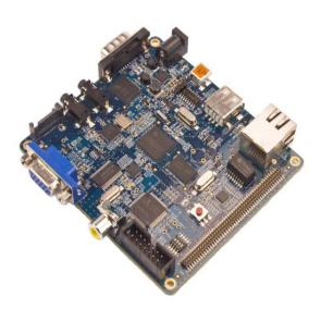
this platform. Inbuilt MMC/SD controller provides an instant add on storage for personal collections. UPP provides a high speed parallel interface to FPGAs & other data converters. Two USB ports provide wide variety of peripheral connectivity. The USB OTG port also provides an option to power the Hawk board when connected to a PC/LAPTOP.
