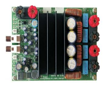
configure the two BTL channels into one parallel BTL (PBTL) channel. The OPA1632 is a High Performance Fully Differential Audio Op Amp designed to allow operation with single ended or differential input signals to the EVM. This EVM stuffed with either TAS5613PHD is a complete stereo analog input power amplifier ready for evaluation and great music.
