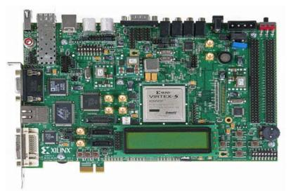
The Virtex-5 FXT platform contains an embedded PowerPC 440 processor block with integrated DMA engines and a multi-port crossbar switches that offers designer's unparalleled FPGA processing power through the ML507. It utilizes Xilinx XC5VFX70T-1FFG1136 Virtex 5 FXT Fpga where the user Users can obtain a quick understanding of the features offered by the ML507 Board.
