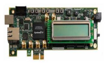
The Cyclone IV GX transceiver starter board is especially suitable for cost-sensitive applications that require high-speed transceivers and power integrity solutions.
