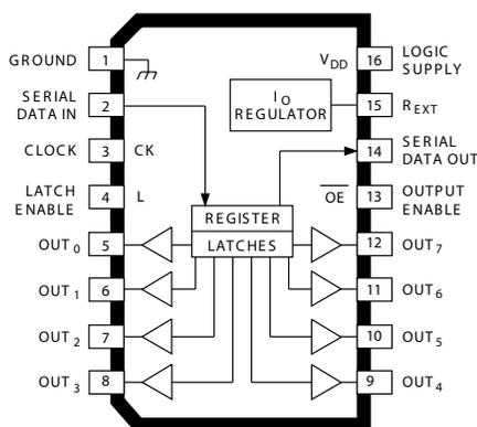
Note that the A6275EA (DIP) and the A6275ELW (SOIC) are electrically identical and share a common terminal number assignment.
