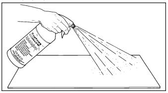
Figure 2. Applying Reztore™ Topical Antistat to the mat
