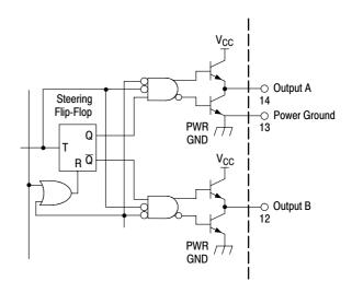
Figure 18. Steering Flip-Flop and Output Drivers
