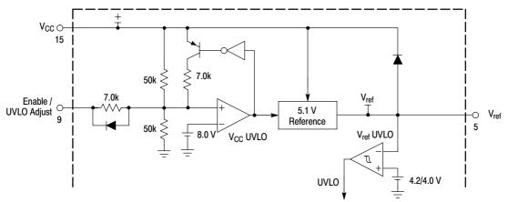
Figure 19. Undervoltage Lockout and Reference
