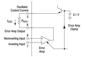
Figure 17. Error Amplifier and Clamp
