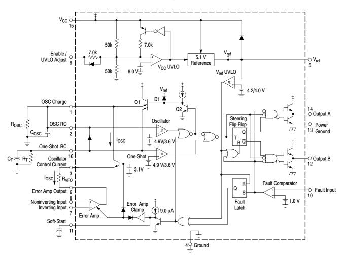
Figure 14. MC34067 Representative Block Diagram
