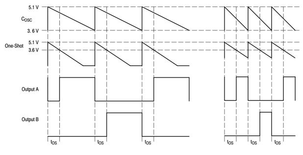
High State Error Amp output, minimum  $I_{OSC}$  current occurring at minimum input voltage, maximum load.
