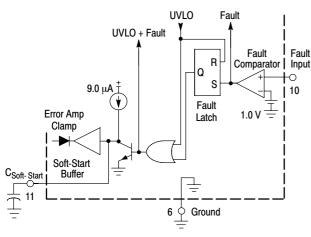
Figure 20. Fault Detector and Soft-Start
