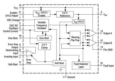
Figure 1. Simplified Block Diagram
