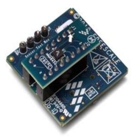
Software is available for download to use with the RD3924MMA8450Q (or separately purchased LFSTBEB8450 and LFSTBUSB). The GUI software providing real time data and demonstration of the latest embedded accelerometer features such as the High Pass Filter, 32 data point FIFO buffer, enhanced Orientation (Portrait/Landscape) detection, Shock Detection, Tap Detection and Transient detection.
