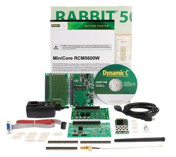
A Development Kit offers the essential hardware tools and includes the Dynamic C® software development system. The Kit contains a prototyping and interface board with USB connections that will allow you to evaluate and debug the RCM5600W.
