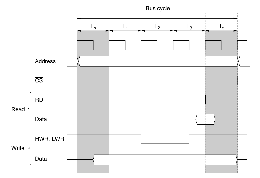
Figure 6.3 \overline{CS} and Address Assertion Period Extension (Example of 3-State Access Space and RDN_n = 0 )
