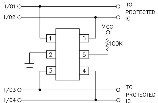
**Data Line Protection Using Internal TVS Diode as Reference**
