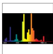
Reference: DULUX EL LL 7 W/41-827 E 27 Rated wattage [W]: 7 220-240/50-60 Supply voltage [V/Hz]: Current Effective value [mA]: 70 LUMILUX INTERNA® Light colour: Colour rendering group [ - ]: 1 B Luminous flux [lm]: 400 Diameter d [mm]: 45 Length I [mm]: 129±3 Weight [g]: 70 Base: E27 Standard pack [pcs]: 10
