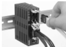
Unit connectors can be used with 16-points and 32-points units. Due to the loose-wiring, pressure contact type design, wiring is easy without the need for insulation. (MIL-C-83503)
