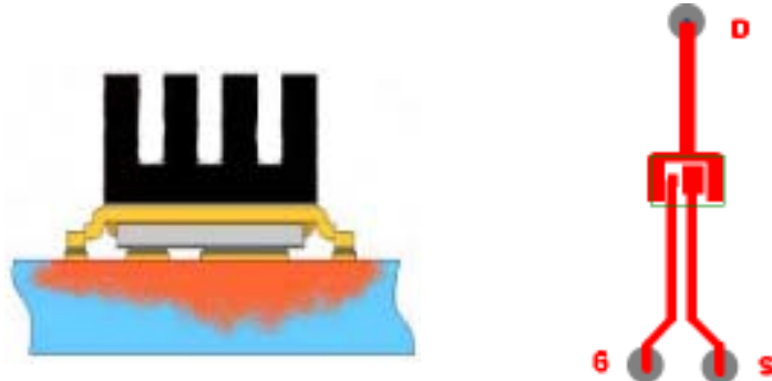
⑩ Mounted on minimum footprint full size board with metalized back and with small clip heatsink. (still air)
