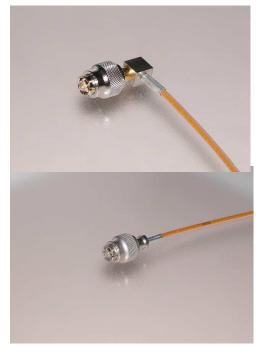
The quick engage / release mechanism is the unique feature in the new Snap Lock Series. Replacing the threaded coupling mechanism with a true snap on interface allows for more connectors in a given space and reduces installation errors. The Snap Lock SMA plugs mate with standard SMA jack making them adaptable to both new and existing systems
