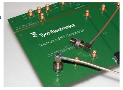
TE Snap-Lock Series SMA plugs are designed to replace standard SMA plugs in existing or new designs. The problem with standard SMA plugs is that they have a threaded coupling mechanism which requires a specific torque (typically 7-10 in-lbs or 0,7–1,1 Nm) for optimum connections. This process takes time, involve wear on the mating component and many times requires a separate tool to ensure that the required torque is achieved.
