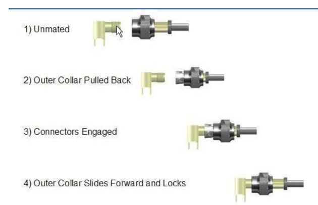
The above diagrams illustrate the ease with which the Snap Lock SMA is mated and unmated. The Snap Lock connector has inner contact fingers which slide over the thread of the mating Jack and lock into place by engaging the outer collar. Disengagement is achieved by pulling back on the outer collar. This design reduces wear on the component and saves application time.
