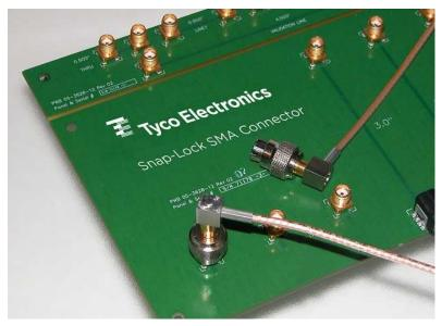
General material and finish specifications of the Snap Lock SMA connector are listed here. Some of the performance characteristics do not include the durability rating of 500 cycles, 50 Ohm impedance and operating frequency up to 11 GHz, matching standard SMA connector performance. The Snap Lock Series is RoHS compliant with gold plated mating surfaces.
