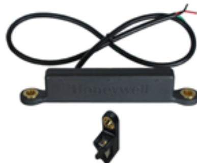
The MR array measures the output of the MR sensors mounted along the magnet's direction of travel. The output and the MR sensor sequence determine the nearest pair of MR sensors to the center of the magnet location. The output of these two MR sensors is then used to determine the position of the magnet between them.
