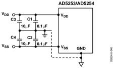
Figure 40. Power Supply-Bypassing Configuration
