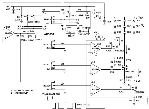
Figure 45. Digital Potentiometer-Based RGB LED Controller
