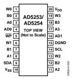
Figure 2. Pin Configuration
