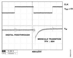
Figure 19. Clock Feedthrough and Midscale Transition Glitch
