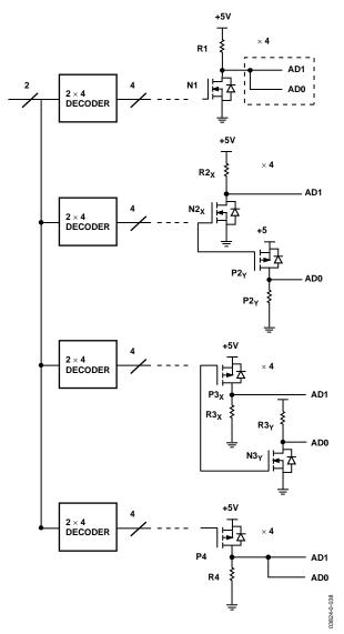
Figure 38. Four Devices with AD1 and AD0 of 00
