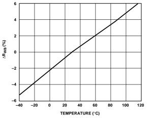
Figure 10. Change of  $R_{WB}$  vs. Temperature
