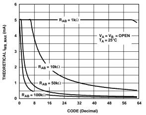
Figure 21. AD5253 IwB\_MAX vs. Code
