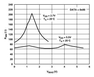
Figure 9. Wiper Resistance vs. V<sub>BIAS</sub>
