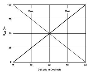
Figure 43. AD5253 R<sub>WA</sub>(D) and R<sub>WB</sub>(D) vs. Decimal Code
