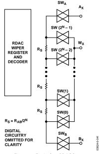
Figure 41. Equivalent RDAC Structure
