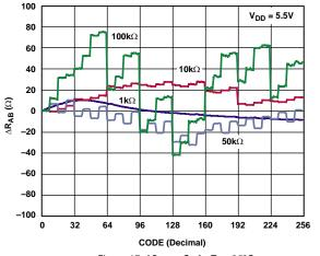
Figure 17.  $\Delta R_{AB}$  vs. Code,  $T_A = 25$ °C
