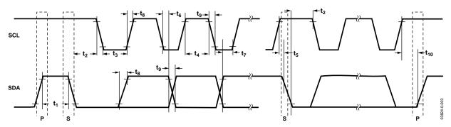
Figure 23. I<sup>2</sup>C Interface Timing Diagram
