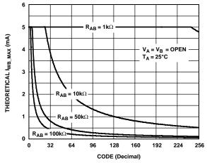
Figure 22. AD5254 IwB\_MAX vs. Code
