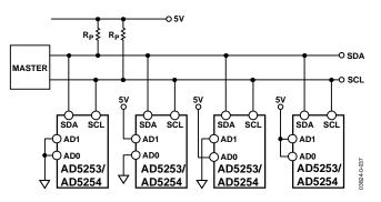
Figure 37. Multiple AD5253/AD5254 Devices on a Single Bus
