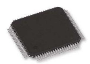
applications. Additional peripherals, such as a 12-bit A/D converter, 3 comparators H/W RTCC, 8 total CCP/ECCP channels, 8 total timers and 69 general purpose I/O, give this cost-effective microcontroller seemingly limitless possibilities in a variety of applications where high performance with low cost is required.
