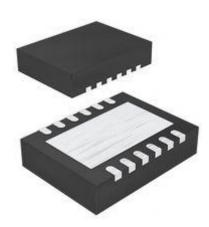
The bq27541 also features integrated support for secure battery pack authentication, using the SHA-1/HMAC authentication algorithm.
