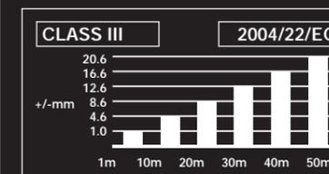
Tools such as tapes that do not carry a class marking may be less accurate, and so could cause problems where high tolerances are required.
