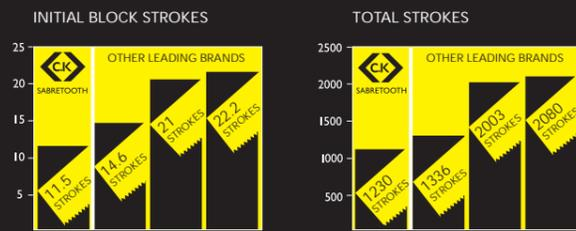
First fix saw tested against UK's market leading saws in independent CATRA tests.
