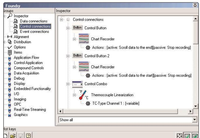
**Figure 12.** Use the Inspector tool to view the control connections of an application.
