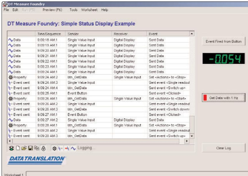
Figure 13. Analyze a running program using the Status Display panel.
