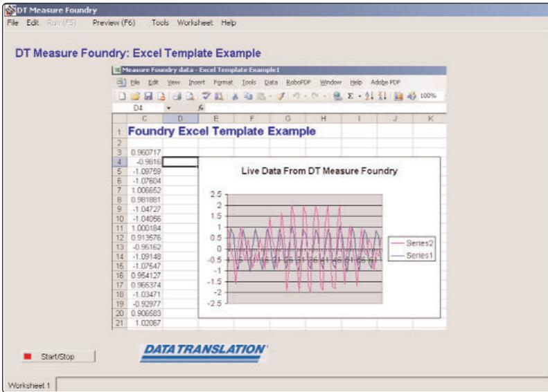
**Figure 9.** Send data directly from DT Measure Foundry to Excel with the Excel Live Link panel. See your Excel spreadsheet change as values are acquired in DT Measure Foundry.
