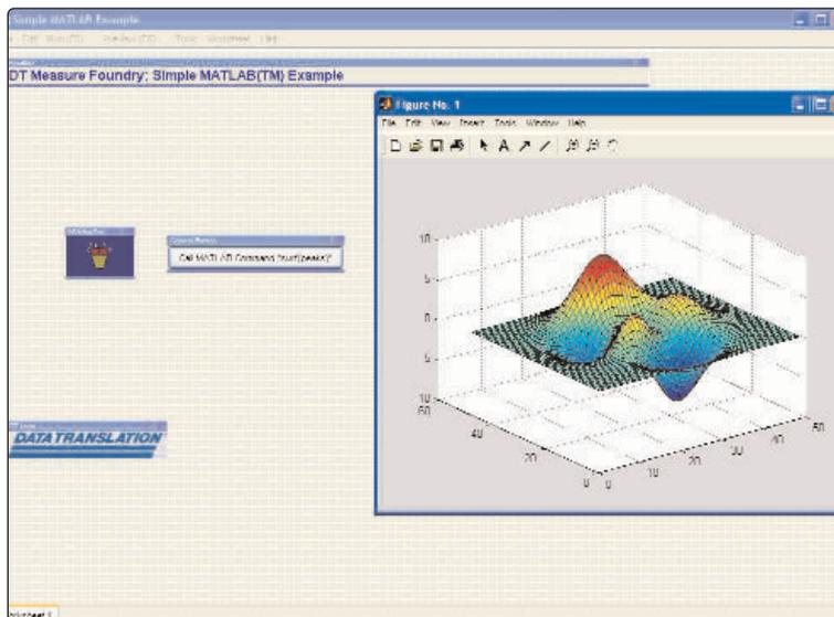
Figure 8. Use MATLAB with DT Measure Foundry to analyze your data. You can perform any MATLAB command or operation within DT Measure Foundry using the Melting Pot panel to exchange data with a MATLAB application.
