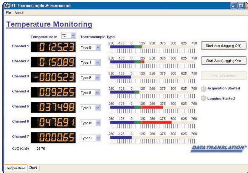
**Figure 6.** Use control panels to control the flow of data in your application. For example, control panels are used above to change the thermocouple type or start and stop your acquisition.
