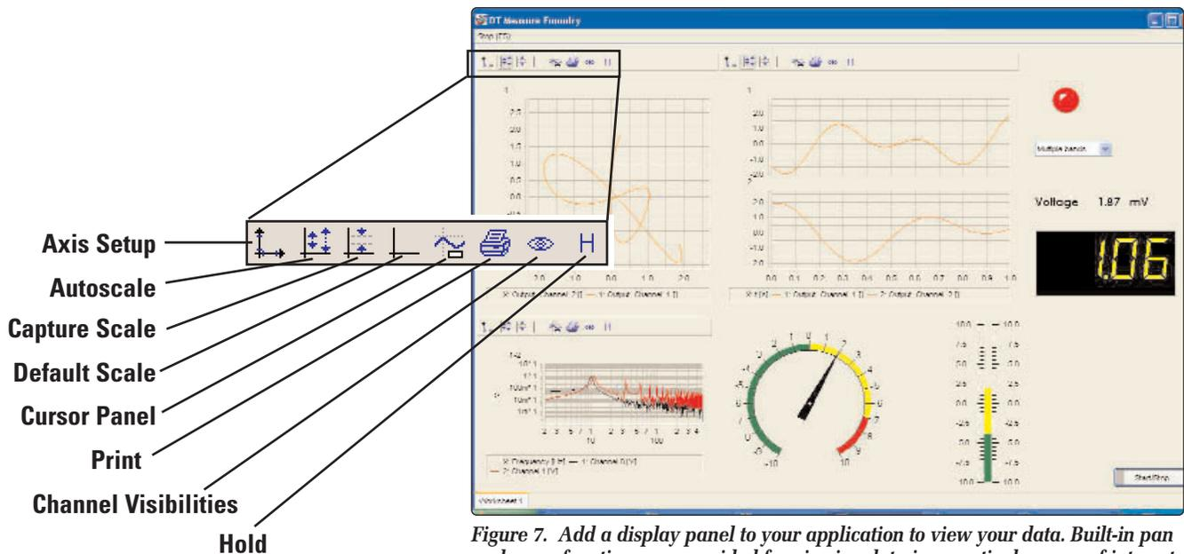
**Figure 7. Add a display panel to your application to view your data. Built-in pan and zoom functions are provided for viewing data in a particular area of interest. You can configure the display as you like, including changing its size, color, and font.**
