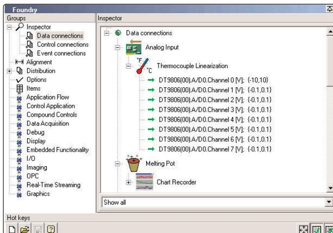
**Figure 11.** Use the Inspector tool to view the data connections of an application.
