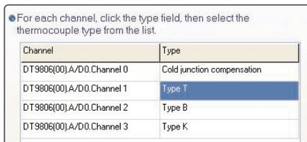
**Figure 4.** The Thermocouple Linearization panel, used here, shows how to use property pages to configure your operation.
