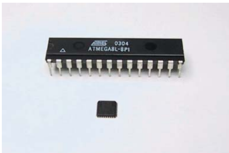
Fig. 3.1.: Comparison of the largest and smallest case in which the ATmega8L chip is available.
