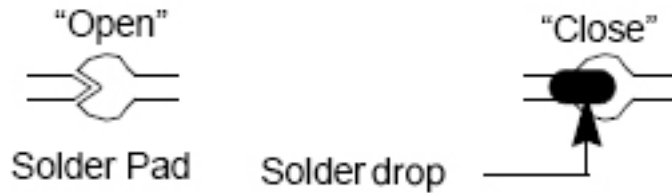
Figure 2-4. Solder Strap Definition
