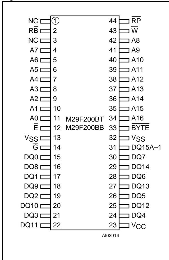
Figure 4. TSOP Connections
