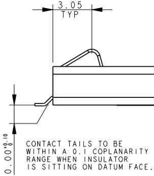
CONTACT TAILS TO BE WITHIN A 0.1 COPLANARITY RANGE WHEN INSULATOR IS SITTING ON DATUM FACE.
