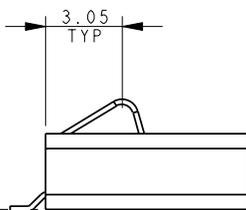
CONTACT TAILS TO BE WITHIN A 0.1 COPLANARITY RANGE WHEN INSULATOR IS SITTING ON DATUM FACE.
