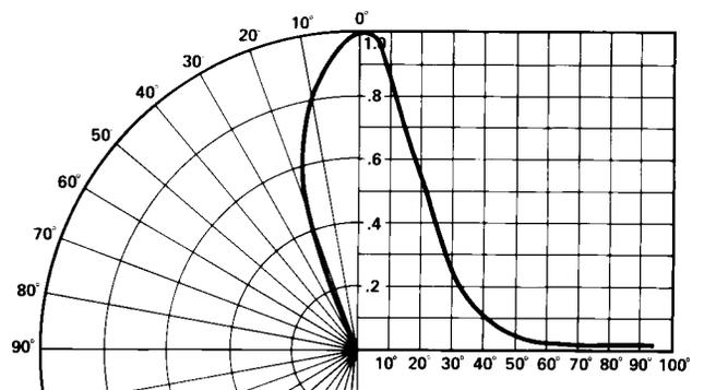
Figure 10. Relative luminous intensity vs. angular displacement.
