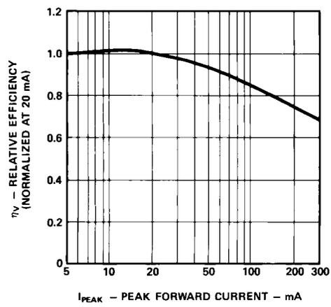
Figure 4. Relative efficiency vs. peak forward current.
