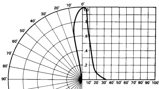
Figure 9. Relative luminous intensity vs. angular displacement.
