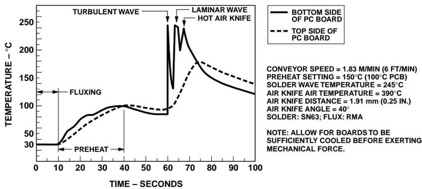
Figure 11. Recommended wave soldering profile.
