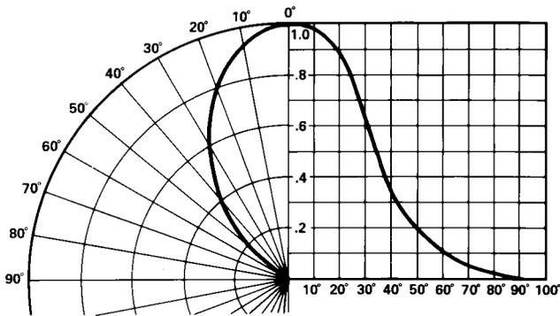
Figure 7. Relative luminous intensity vs. angular displacement.
