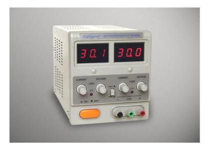
The *digimess*® BP3002 is a low cost general purpose linear dc power supply unit with both plus and minus outputs. The power supply can operate in either constant voltage or constant current modes and features large red LED displays for both voltage and current. Short circuit and current limit protection are included and the BP3002 is supplied with a mains lead and an operating manual.
