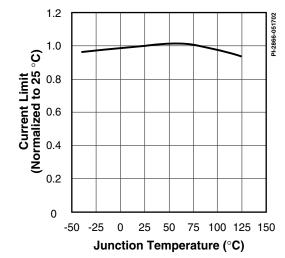
Figure 37. Internal Current Limit vs. Temperature.
