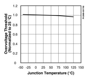
Figure 39. Overvoltage Threshold vs. Temperature.
