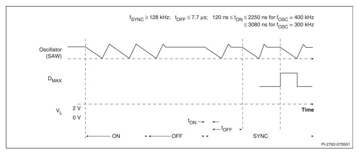
Figure 6. Synchronization Timing Diagram.
