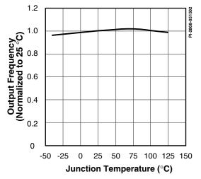
Figure 36. Frequency vs. Temperature.
