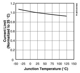
Figure 38. External Current Limit vs. Temperature with  $R_{\mu} = 12 \ k\Omega$ .
