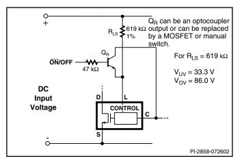
Figure 22. Active-off Remote ON/OFF with LINE-SENSE.
