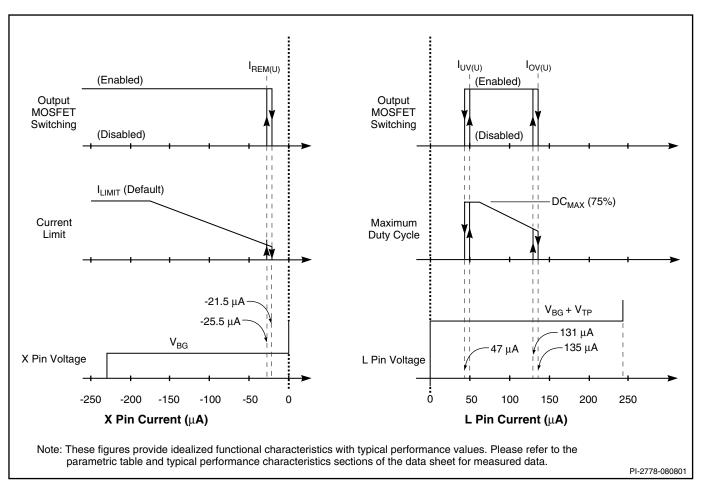
Figure 7. LINE-SENSE and EXTERNAL CURRENT LIMIT Pin Characteristics.
