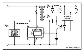
Figure 1. Typical Forward Converter Application.
