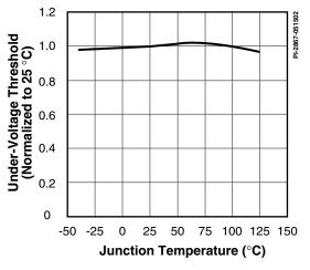
Figure 40. Under-Voltage Threshold vs. Temperature.
