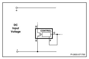
Figure 9. 400 kHz Frequency Operation.
