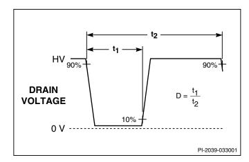
Figure 30. Duty Cycle Measurement.
