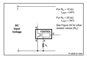
Figure 15. Externally Set Current Limit.
