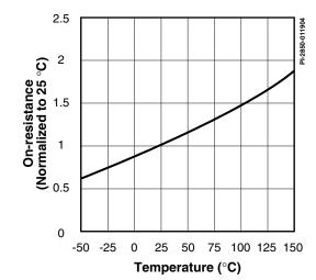
Figure 49. On-Resistance vs. Temperature.
