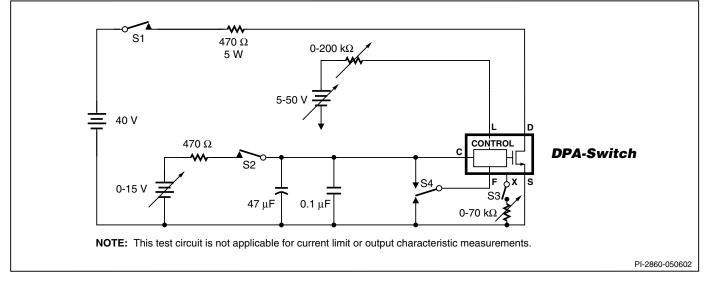
Figure 33. DPA-Switch General Test Circuit.
