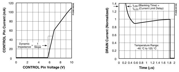
Figure 31. CONTROL Pin I-V Characteristic.
