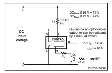
Figure 21. Active-on Remote ON/OFF with LINE-SENSE and EXTERNAL CURRENT LIMIT.
