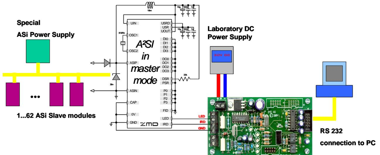
**Maximum digital voltage level at CMOS input and output port is limited to 5V DC!!!**
