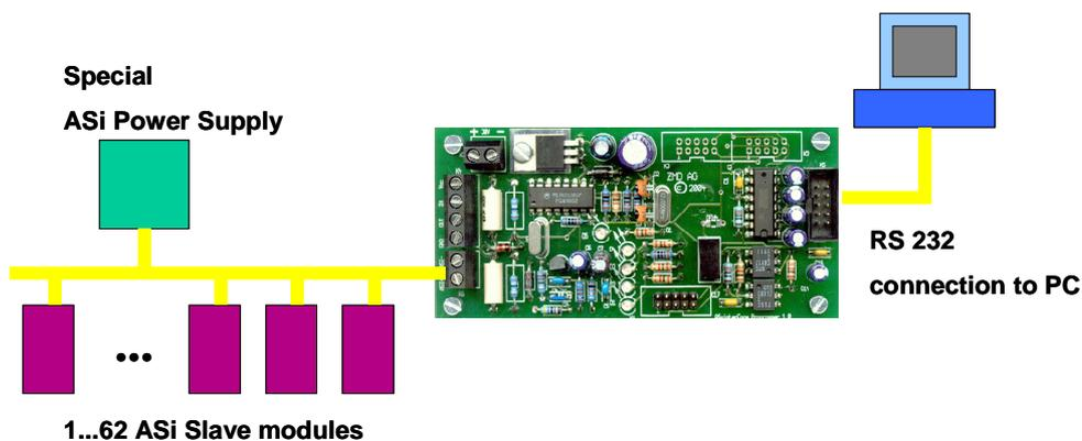
The power supply of the complete system, including ASi modules and ASi programmer will be provided by a special AS-interface power supply. No additional power supply at the 30V connector is allowed.
