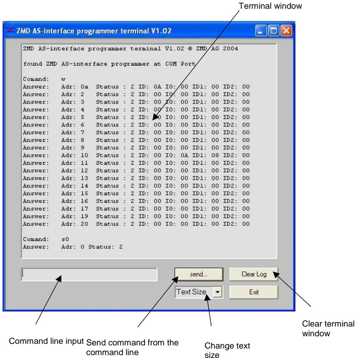
1. Type a valid command in the command line. For example “d12 2” – data exchange to slave with address 12 , send data 2 (decimal).
