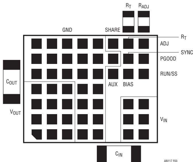
**Figure 3. Moving the  $C_{OUT}$  Capacitor Away from  $C_{IN}$  Can Reduce Output Noise**
