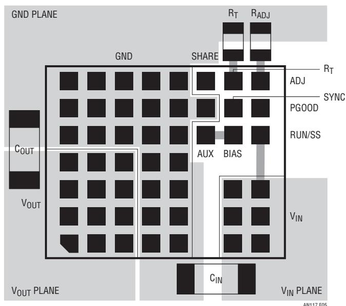
**Figure 5. Suggested Power and Ground Planes for LTM8023. Note the Wide Gap that Separates the High Voltage  $V_{IN}$  net From Other Nets, in Compliance with IPC-2221**
