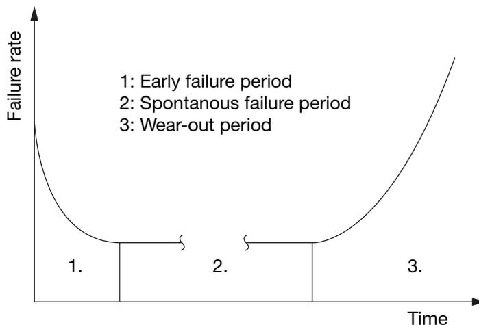
For the sake of simplicity, the first two phases are combined into a so-called “extrinsic reliability period”. The third phase, the wear-out period, is correspondingly designated as the “intrinsic reliability period”.
