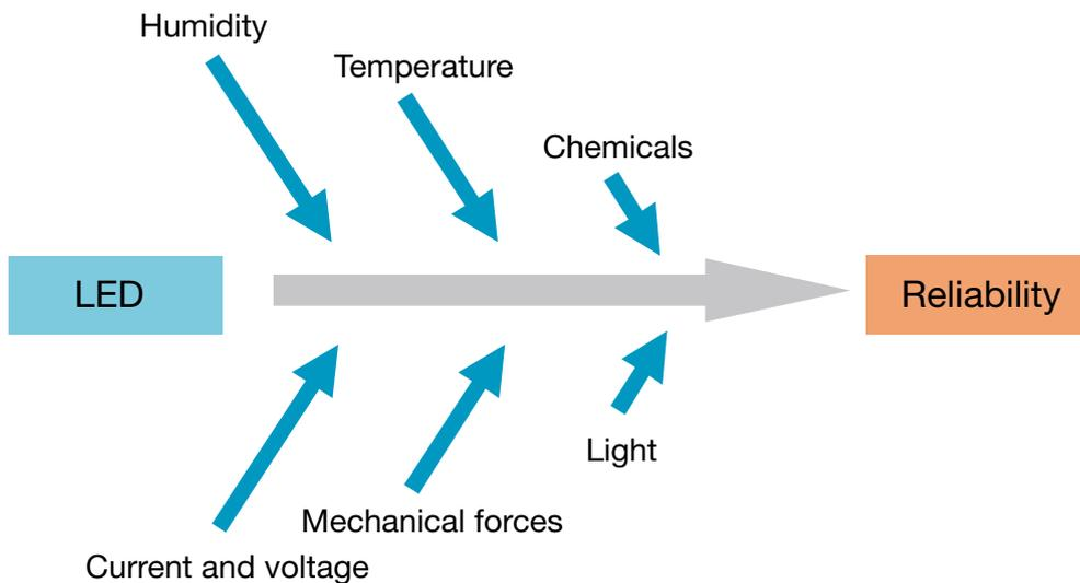
These can even lead, in a worst case situation, to a total failure or influence the aging characteristics in the long term (e.g. brightness), and thus produce a change in the reliability and lifetime. Such direct influencing factors are the temperature and resulting junction temperature  $T_{j(\text{unction})}$  of the LED, for
