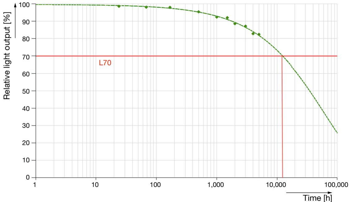
Since aging is based on a change in the material properties and is therefore subject to statistical processes, the lifetime values also are based on a statistical distribution.
