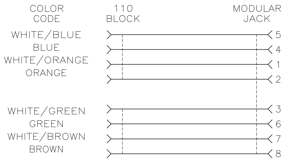
ELECTRICAL SCHEMATIC T568B
